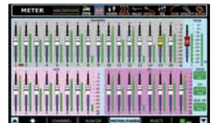
Virtual faders with meter for each input channel, AUX and Group mix
