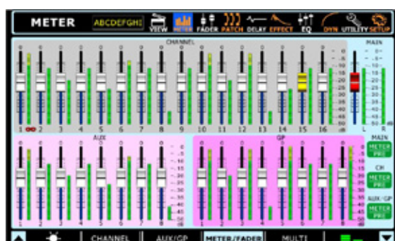
Virtual faders with meter for each input channel, AUX and Group mix
