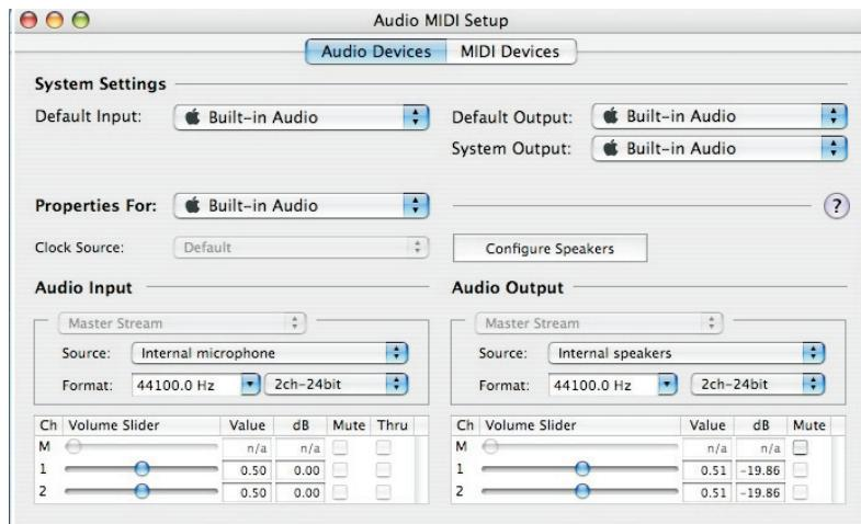
Enter the Audio Devices section. From the "Properties for" pull-down tab, select Helix Board 12 FireWire MKII.
