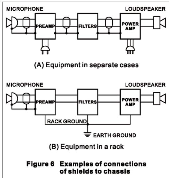
**Figure 6 Examples of connections of shields to chassis**
