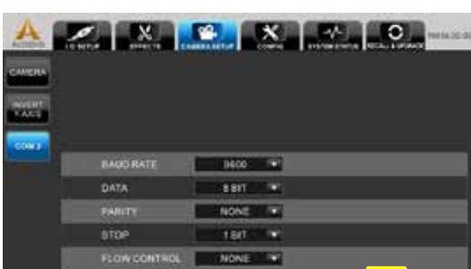
The Com 2 (RS232) Setup remains the same as Camera COM 1 setup, but without the input setting.
