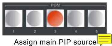
Use PGM cross-point buttons to assign main PIP source. Channel 5 cannot be used.
