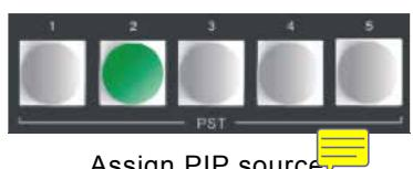
Use PST cross-point buttons to assign PIP sub-source. Channel assigned to DSK cannot be used.
