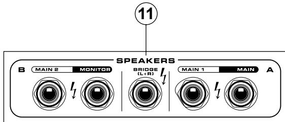
Please note that the Bridge Mono function is only available on the Powerpod 740 models, and is not available on the Powerpod 780 models. With this in mind, we ask customers that own these models to ignore the Bridge connection found in the following speaker setup diagrams.
