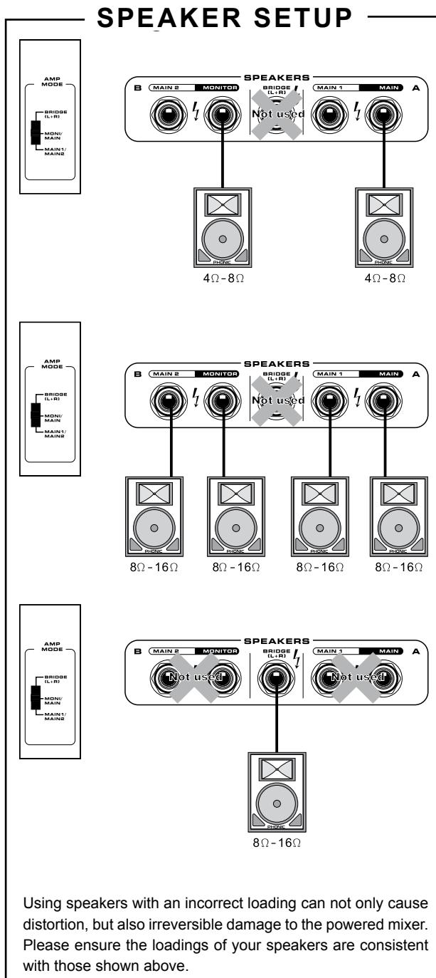
Using speakers with an incorrect loading can not only cause distortion, but also irreversible damage to the powered mixer. Please ensure the loadings of your speakers are consistent with those shown above.
