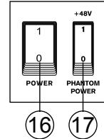
**NB.** Phantom Power should be used in conjunction with balanced microphones. When Phantom Power is engaged, single ended (unbalanced) microphones and instruments should not be used on the Mic inputs. Phantom Power will not cause damage to most dynamic microphones, however if unsure, the microphone's user manual should be consulted.
