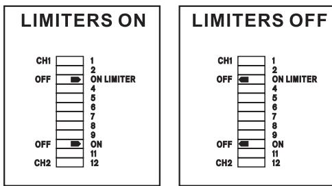
These DIP switches (DIP switches 3 for channel 1 and number 10 for channel 2) allow you to activate the peak limiter circuit built into the power amplifier. This function will reduce distortion and protect speakers. To activate the built-in limiters, DIP switches 3 (channel 1 limiter) and 10 (channel 2 limiter) should be set to the right position.
