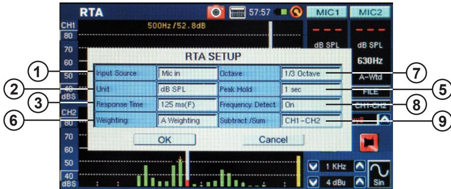
**5. Peak Hold** – The peak hold function will cause the highest signal peaks to be held for a short period of time, giving a better visual representation of these high peaks. This is typically represented by a small red line/dot at the top of the frequency bar. This red mark will remain for as long as the peak hold time is set, or until the frequency's signal rises above the previous peak.
