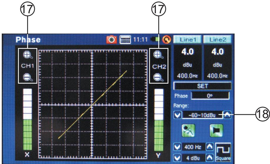
**17. Zoom Icons** – Featured on functions like Phase and Scope, these + and – icons will allow users to zoom in and out on their current results. In the case of the Phase meter, these icons will allow users to zoom in on the X and Y axis of the accompanying graph.
