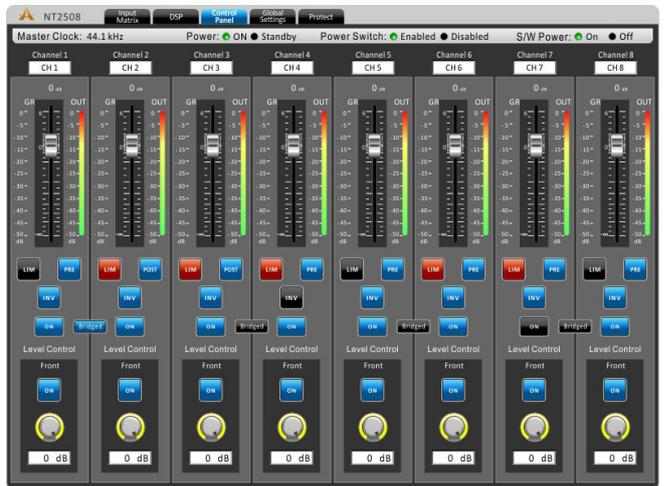
**Limiter:** This button will activate the internal limiter function for the corresponding channel. The limiter can be adjusted through the Global Settings > Lim page.
