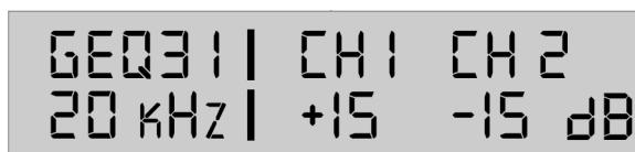
Any GEQ settings can be reset using the “Reset” option. Doing so will return the boost/cut for each frequency of the 31-band GEQ back to 0 dB.
