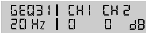
The iAMP DSP features a 31-band graphic equalizer on each of the two output channels. There are, of course, 31 different frequencies between 20 Hz and 20 kHz that can be adjusted by a rate of  $\pm 15$  dB.
